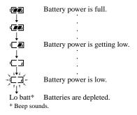
To keep the original battery capacity for a long time, charge the batteries only when they are completely depleted.
